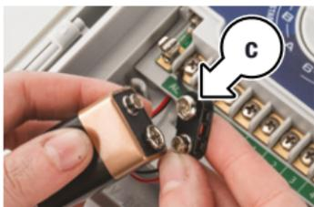
4. Fit in the compartment labelled **9V BATTERY** in the lower end of the housing
