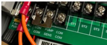
2. Replace with the two wires from the rain sensor into these terminals, polarity NOT required
