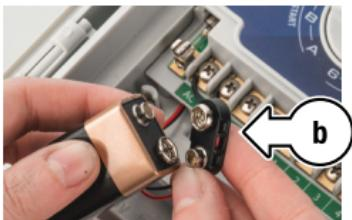
4. Connect a 9V battery to the snap, and fit below the terminal block (c)
